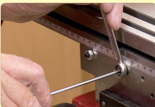
164: Working from the middle outwards, adjust and lock each in turn
