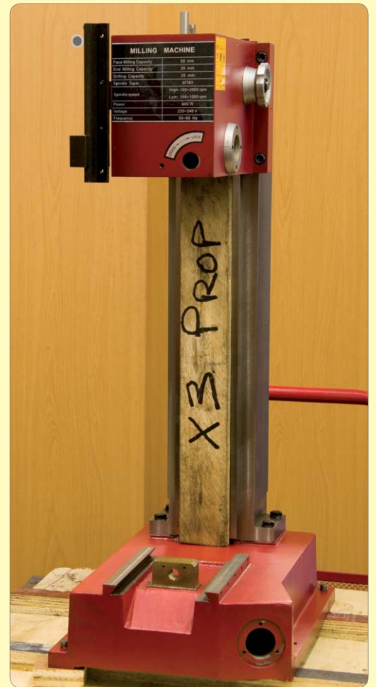
94: X3 Mill stripped, cleaned and ready to assemble
