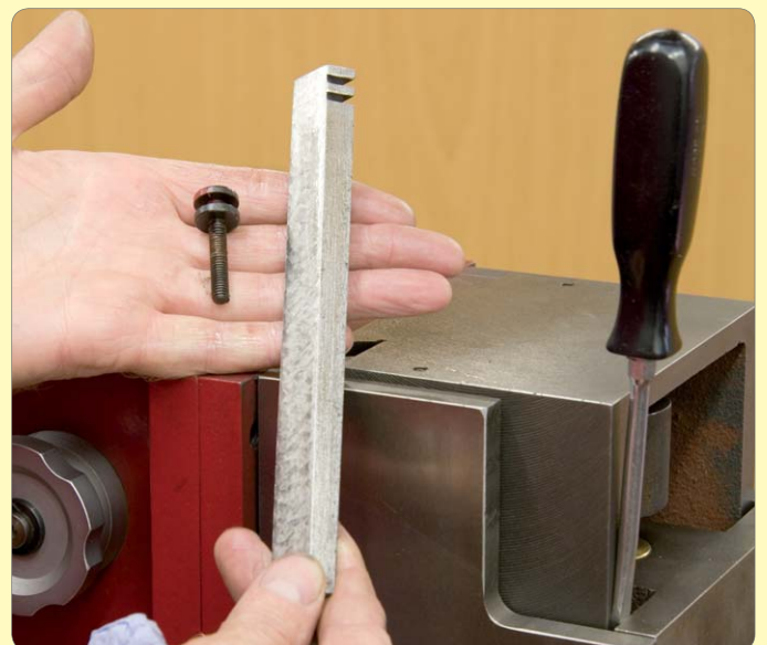
137: Check gib strip is straight and flat, lubricate and re-fit
