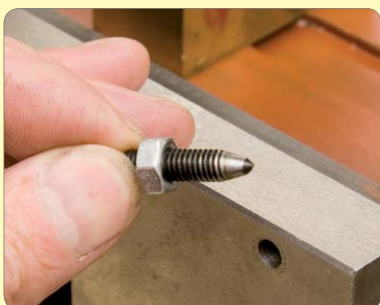
145: Check tips of gib adjusting screws for concentricity
