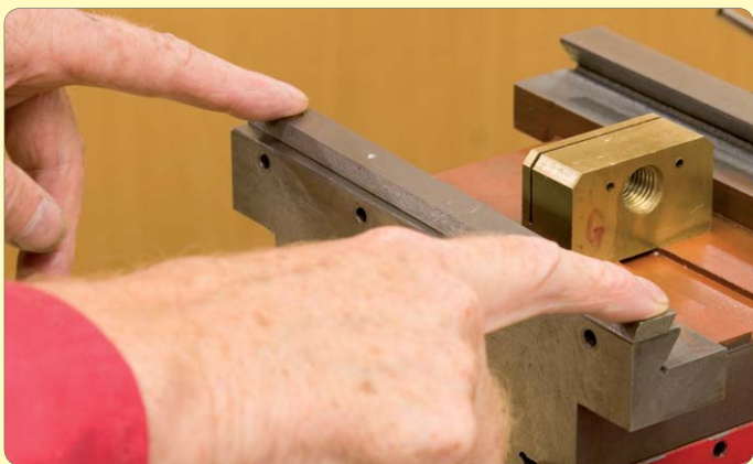
143: Check gib strip is straight and flat
