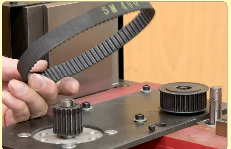
197: Fit driven pulley and belt
