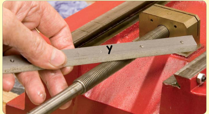
38: Remove and mark Y-Axis gib strip
