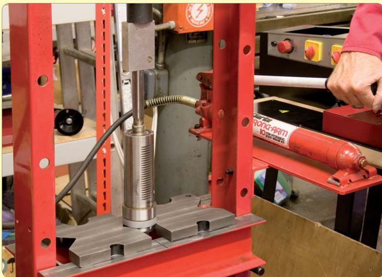
73: Press out inner spindle noting bearing fit as some bearings may be too tight on spindle - this can be adjusted later
