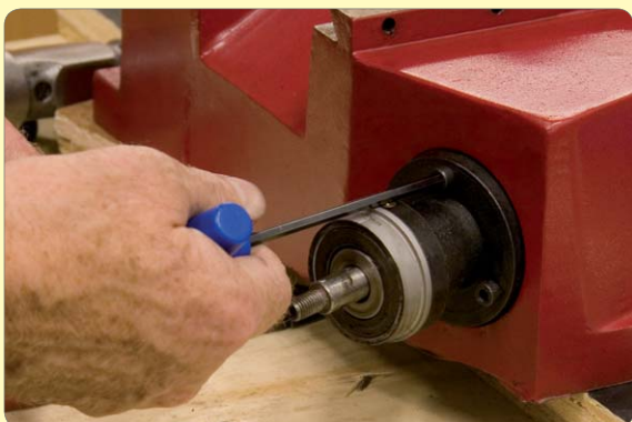
60: Remove screws from bracket
