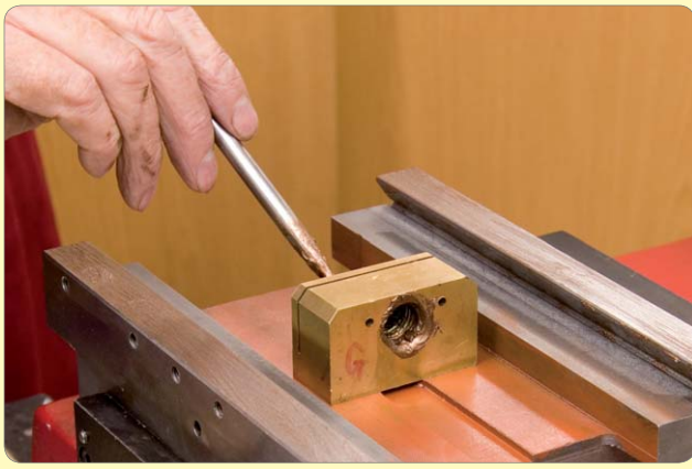
157: Grease table leadscrew nut and dovetails
