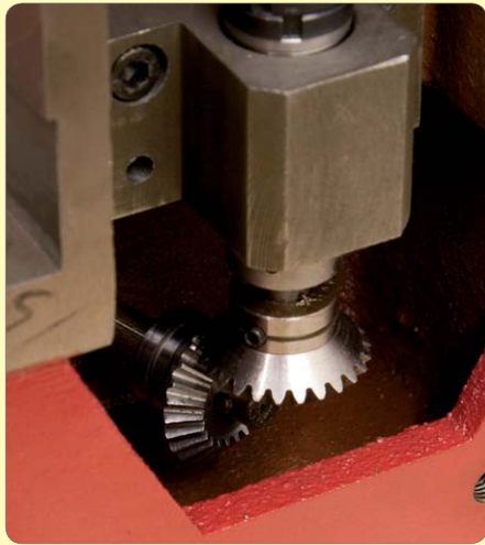
133: Adjust bevel gear mesh and backlash, lock and grease
