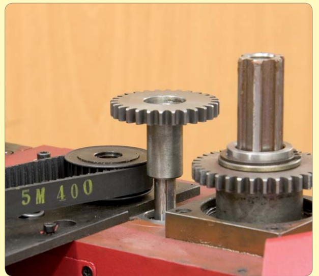
199: Fit reduction box output gear
