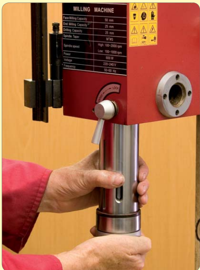
102: Fit spindle aligning guide slot
