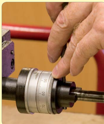
23 : Drive out taper pin through micrometer dial sleeve...
