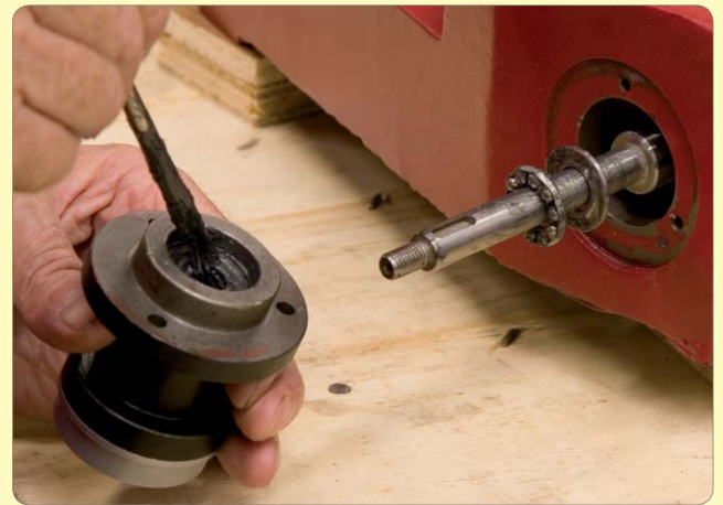
117: Grease and fit thrust race and bearing and grease inner bearing races
