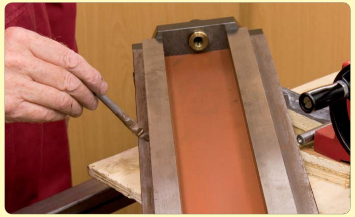
158: Grease table dovetails and leadscrew bush
