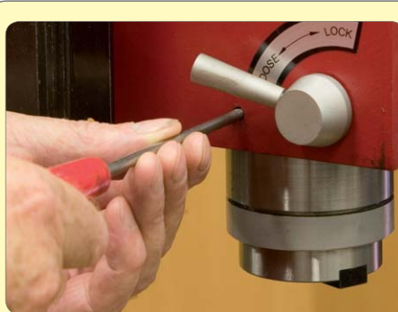
67: Remove first the locking screw...
