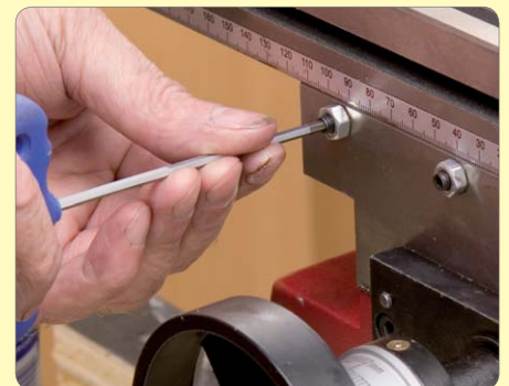
163: Grease and fit adjusting screws
