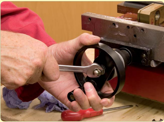
33: Remove Y-Axis handle assembly
