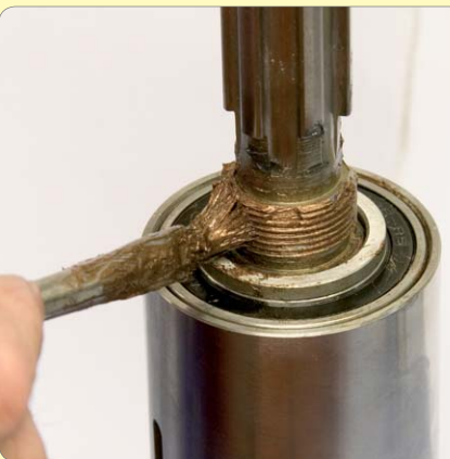
89: Grease threads with Copperslip
