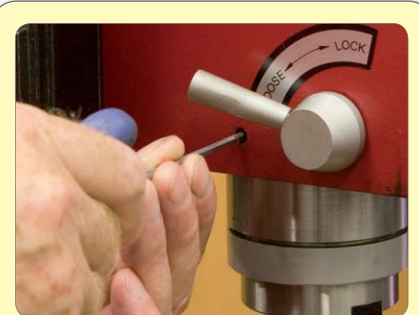
68: ...and second the spindle anti rotation guide pin beneath
