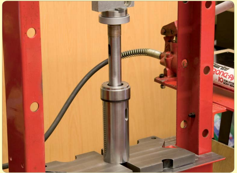
83: Press spindle into spindle sleeve
