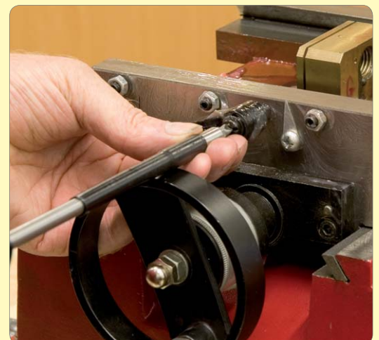
32: Remove table lock, gib adjusting screws and pointer
