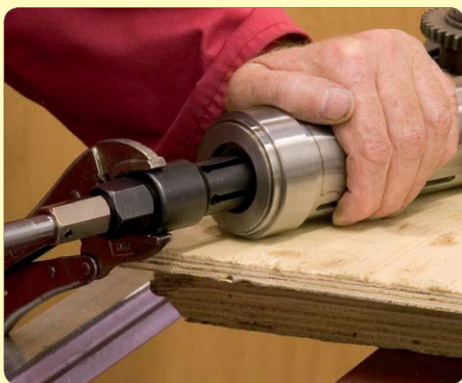
74: Using blind bearing puller, remove taper roller bearing and bearing cover
