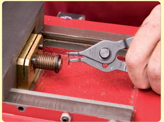
151: Fit washer and circlip at rear of leadscrew
