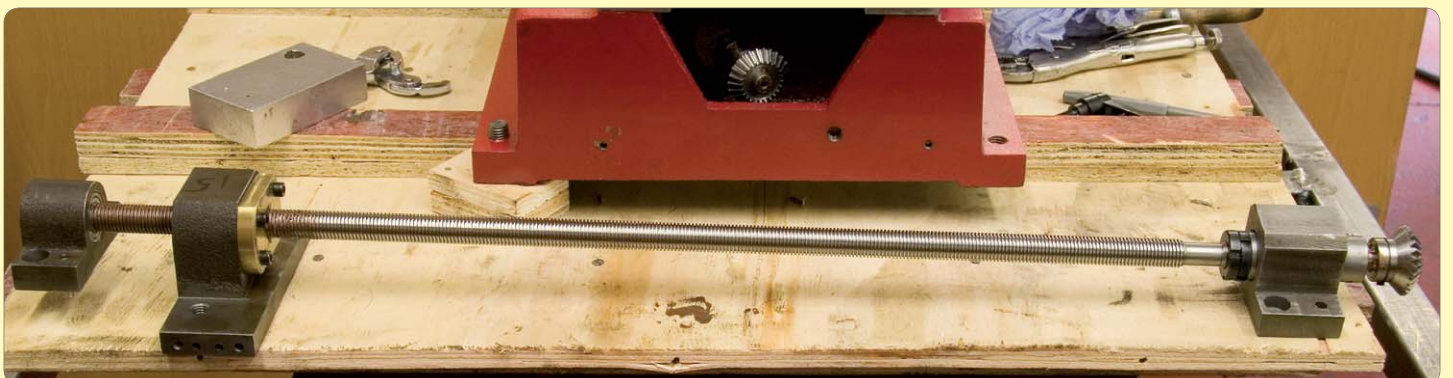
131: Finished Z-Axis leadscrew assembly
