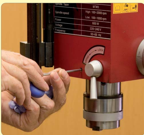
105: Fit anti-rotation grub screw and locking screw
