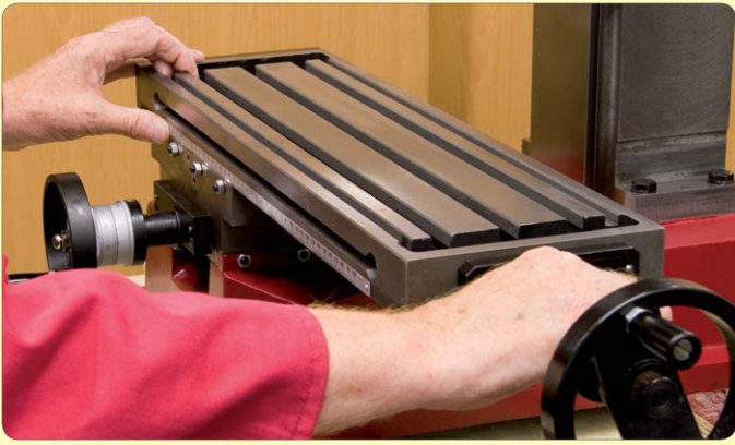
175: Wind table to far right. With thumb on joint between table and saddle, use right hand to move table backwards and forwards to check for slack in dovetails
