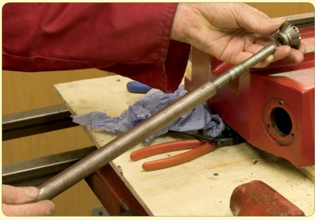
62: Remove shaft and gear at other end
