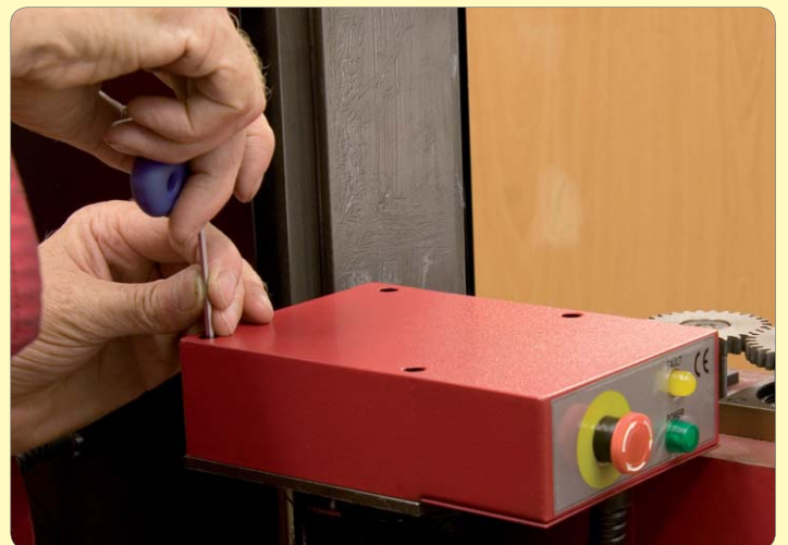
15: Undo emergency stop cover screws 1 turn
