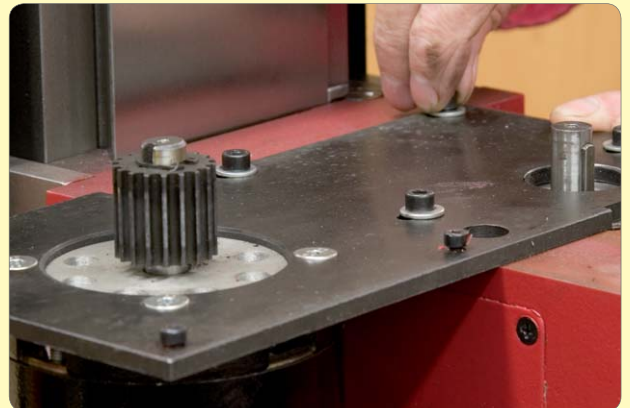
195: Loosly fit motor plate screws
