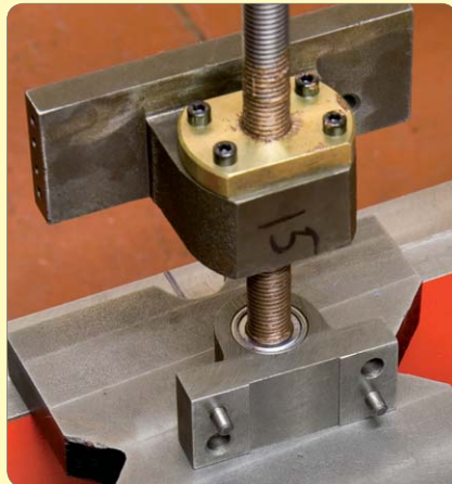
125: Press on Z-Axis top bearing assembly
