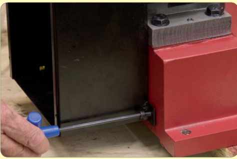
192: Fit 2 lower screws and 2 top casing screws
