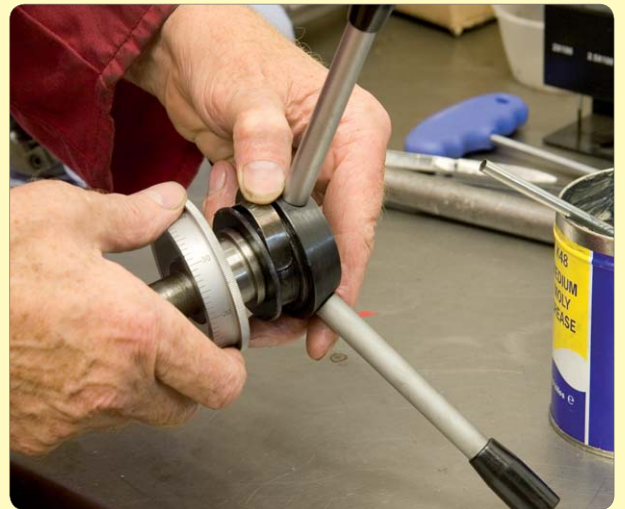
96: Grease and fit micrometer dial and friction spring to handwheel assembly
