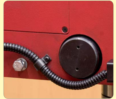
193: Fit guard micro switch and Secure trunking with P-clip
