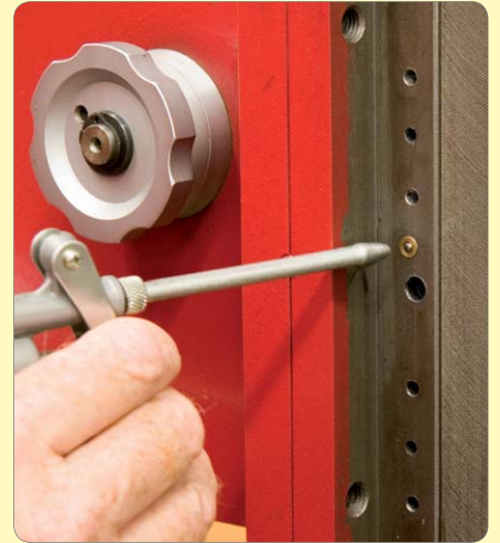
134: Check oilers work
