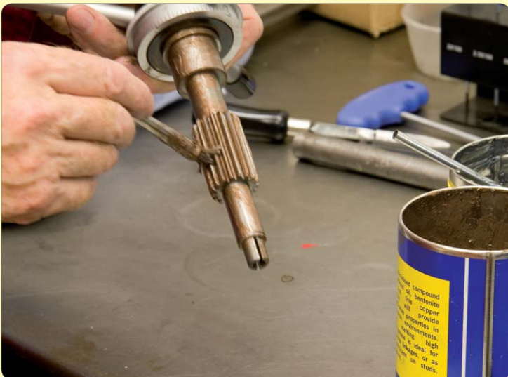
97: Grease splines and shaft on handwheel assembly
