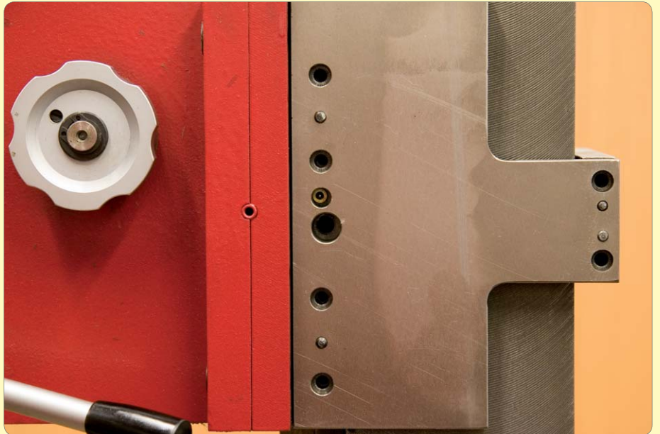
135: Align Z-axis nut with head and temporarily fit sideplates and cap head screws - do not tighten yet. Remove head prop. Tighten head gib strip to lock head position and finally tighten side plate cap screws
