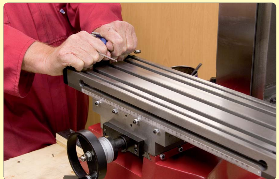
165: Check table movement after each adjustment
