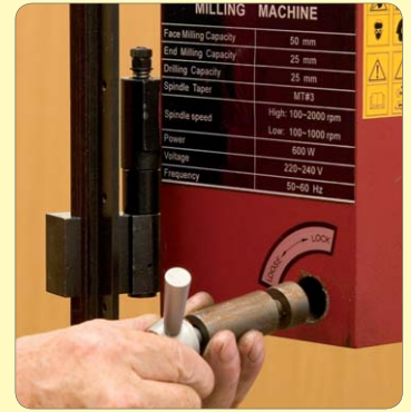
101: Fit spindle lock assembly noting cut-outs for spindle sleeve
