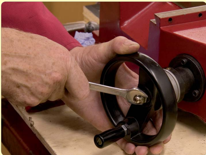
58: Undo adjusting nuts and remove handwheel assembly
