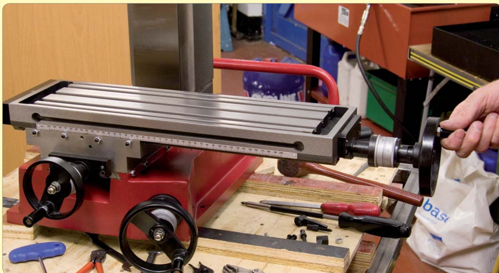
174: Wind table back and forth to check for free movement and minimum drag
