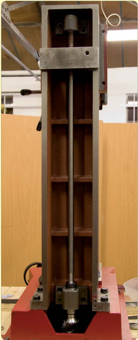
132: Fit Z-Axis assembly to rear of column
