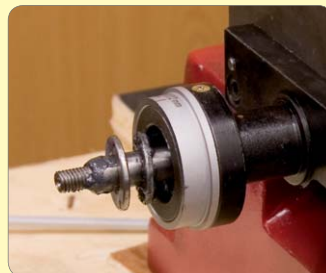
153: Fit outer thrust bearing
