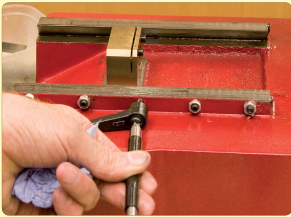
41: Remove locking handle assembly and gib screws
