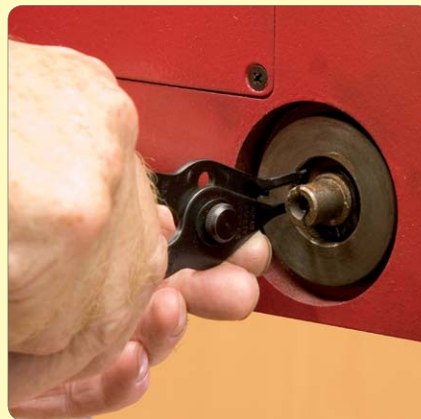
106: Fit spacer and circlip
