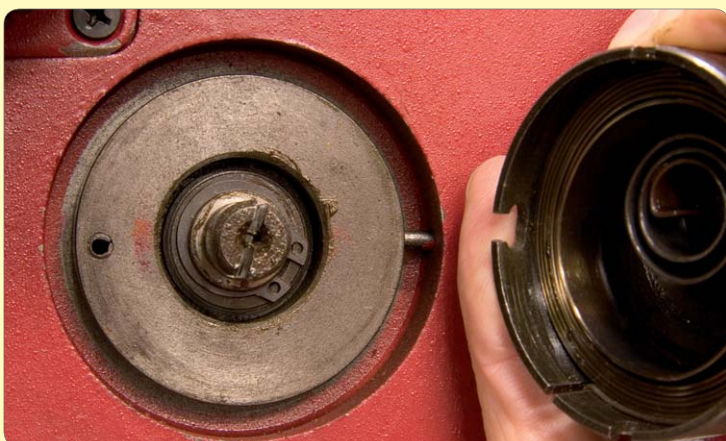
108: Note how end of spring locates in slot and T-slot locates on pin
