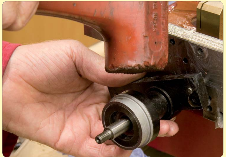
36: Tap off bracket and thrust assembly
