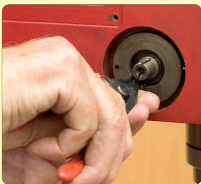
66: Remove circlip and spacer
