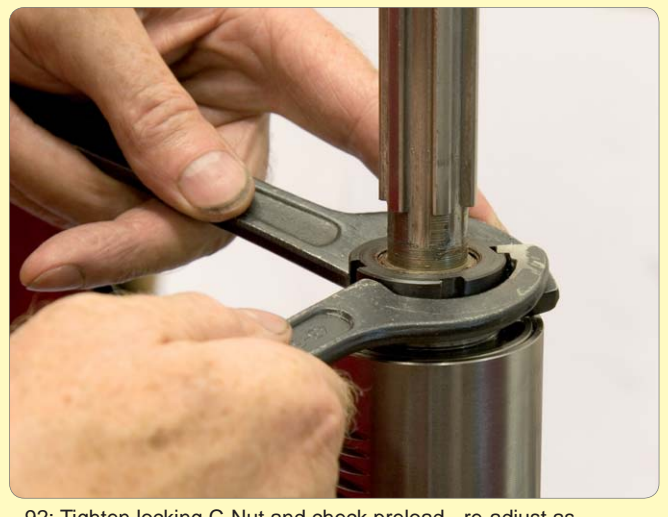
92: Tighten locking C-Nut and check preload - re-adjust as necessary
