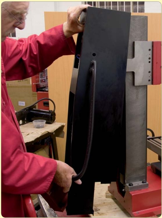
191: Fit rear electronics casing
