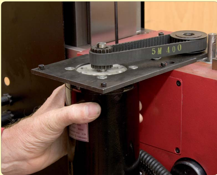
198: Pull motor towards you to tension the belt and lock motor plate screws
