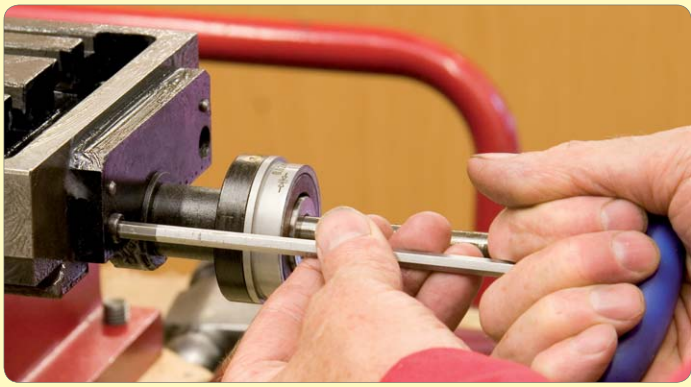
25: Remove leadscrew bracket screws
