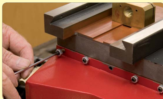
146: Grease and fit adjusting screws
