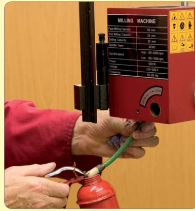
100: Lightly oil bottom of spindle bore
