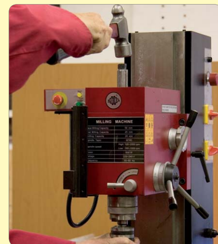
5: ...and give it a tap to release the taper...
