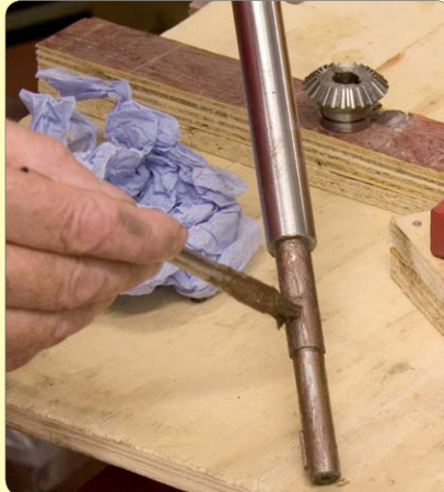
114: Grease Z-axis handle shaft
