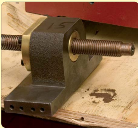
124: Assemble nut noting orientation
