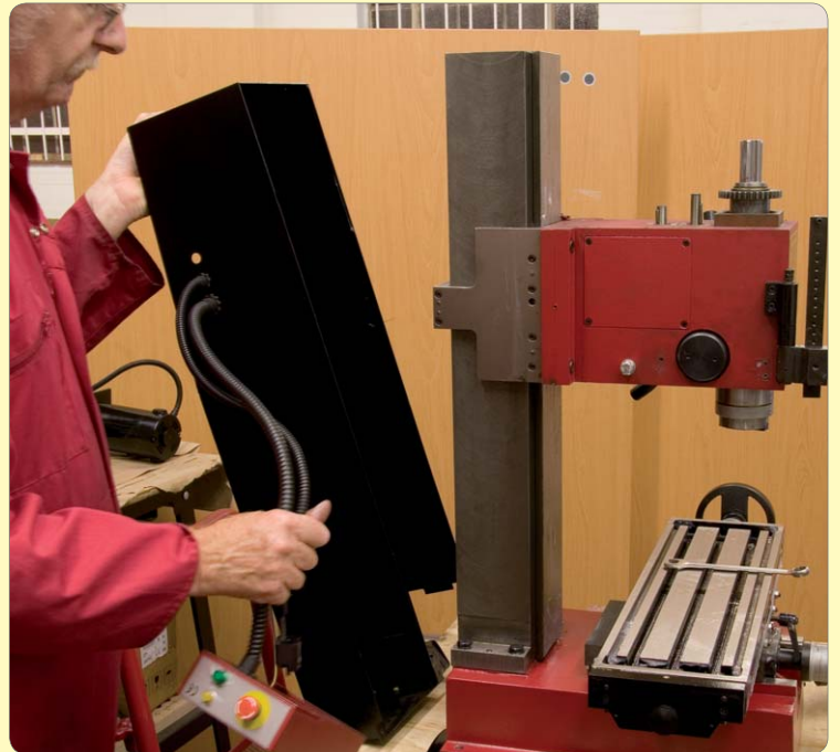
21 : Remove rear control box complete
