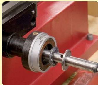
169: Fit outer thrust bearing
