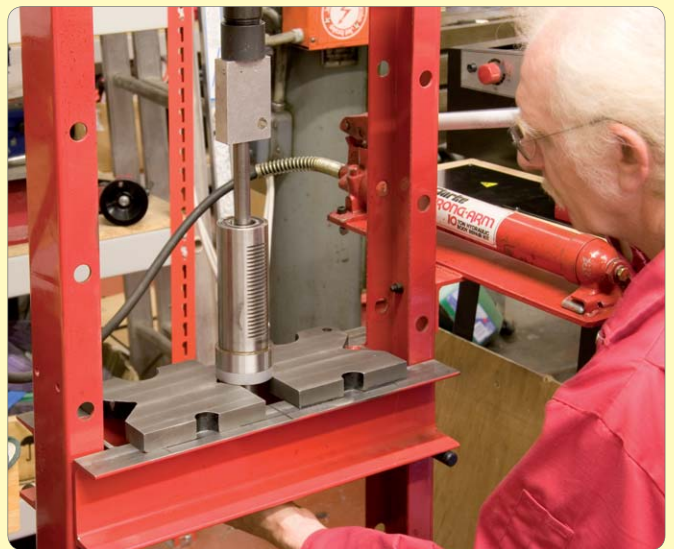
73: Press out inner spindle noting bearing fit as some bearings may be too tight on spindle - this can be adjusted later
