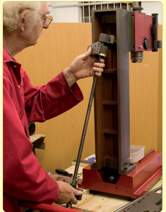
51: Remove leadscrew assembly
