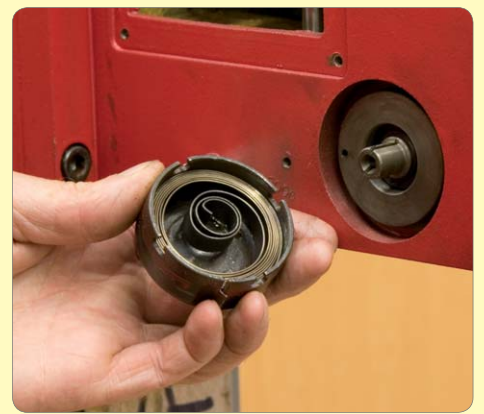
63: Remove gearbox cover
