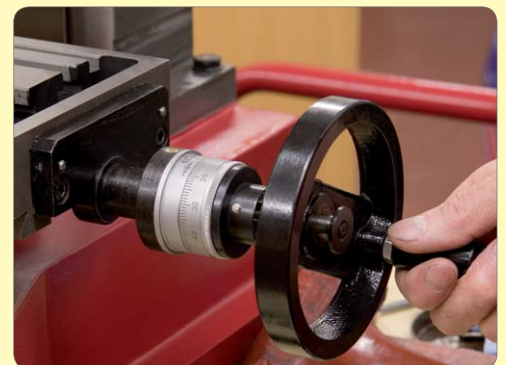
173: Fit handwheel assembly
