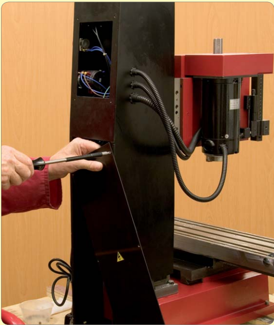
7: Remove rear control panel covers
