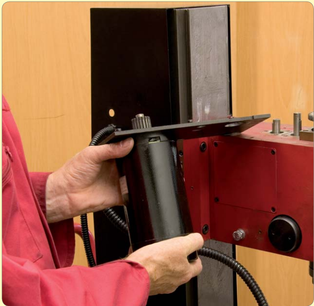
20 : Remove motor and plate
