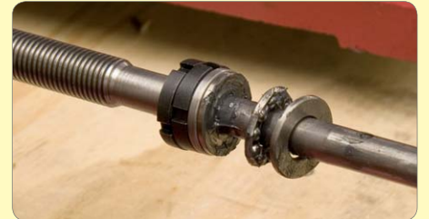
126: Grease and assemble lower block thrust bearing
