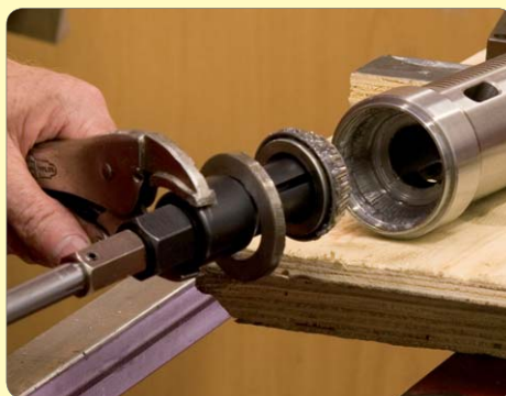
74: Using blind bearing puller, remove taper roller bearing and bearing cover
