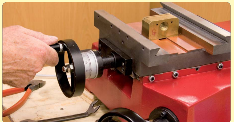
156: Wind saddle in and out to check for smooth and consistent travel making final adjustment to gib strip as required
