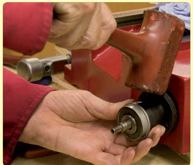
61: Remove carrier bracket and thrust bearings
