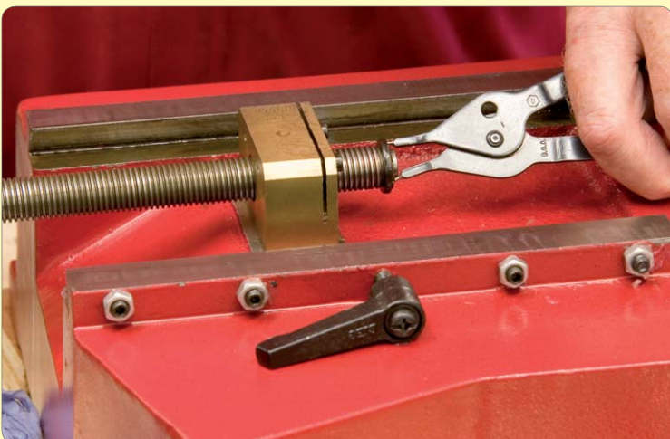
39: Remove circlip and washer from end of leadscrew
