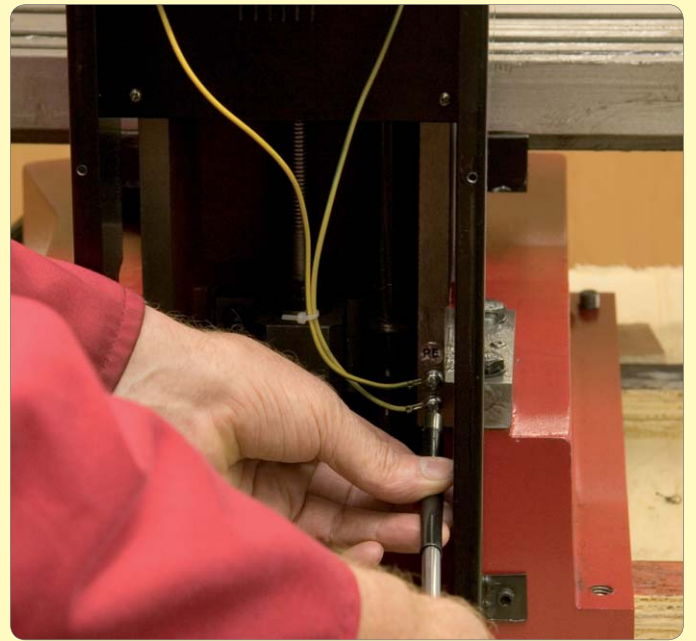
8: Remove earth terminals at base of column
