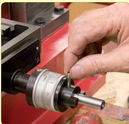
171: Fit sleeve and locate holes for taper pin
