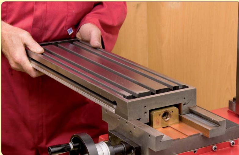
159: Slide table onto saddle
