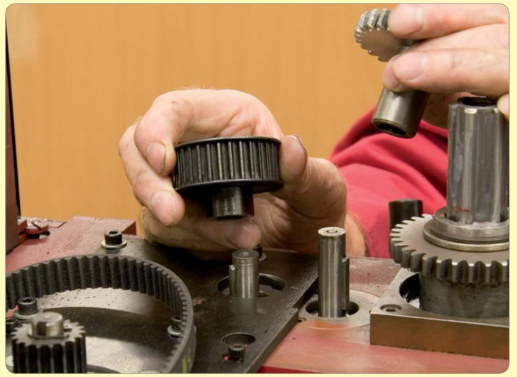
19 : Remove Pulley and gear
