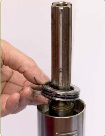
84: Grease and assemble thrust bearing
