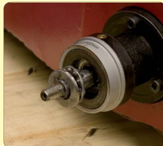
119: Grease and assemble outer thrust bearing and race
