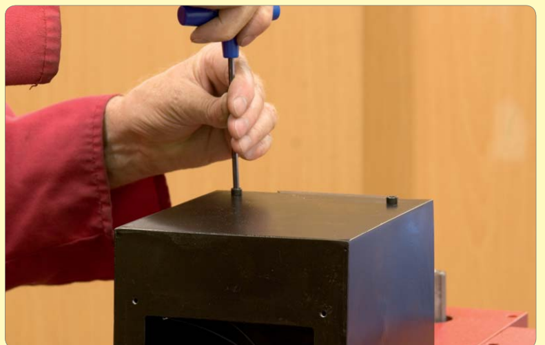
11: Remove 2 cap heads at top & 2 cap heads at bottom of control panel
