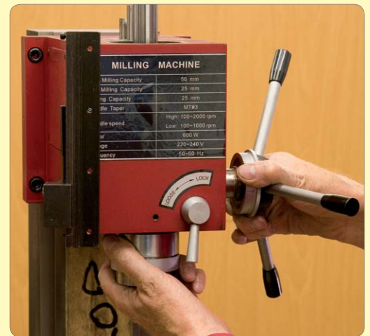
104: Fit handwheel assembly and rotate to desired position
