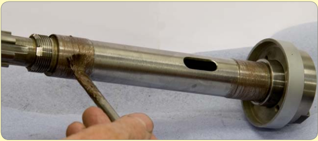
82: Coat bearing journals before assembly with Copperslip grease etc
