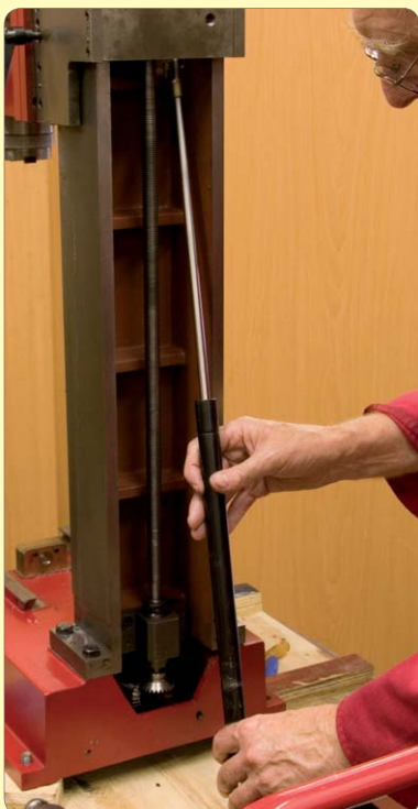
45: Remove gas strut
