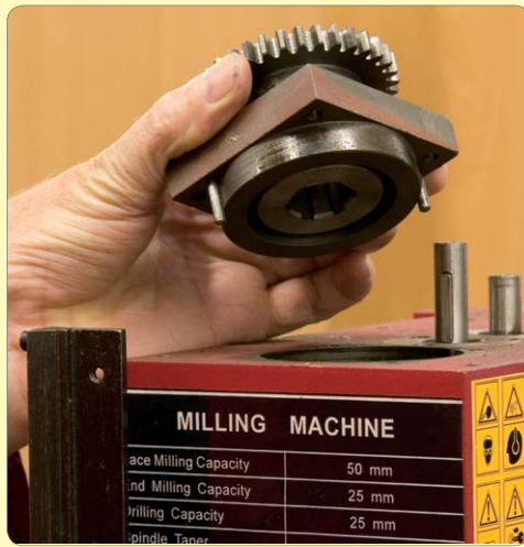
71: Drift out spindle drive gear assembly marking position for later re-assembly
