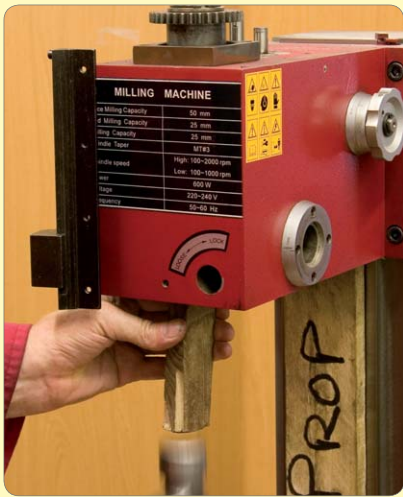
71: Drift out spindle drive gear assembly marking position for later re-assembly
