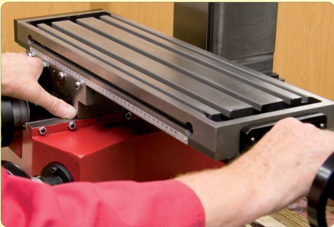
177: Wind saddle fully in and do check again
