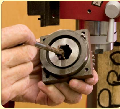
111: Grease drive bearings and gear carrier splines
