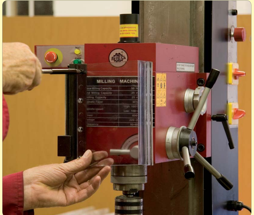
3: Remove the polycarbonate front guard
