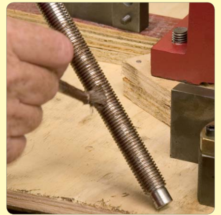
123: Grease Z-Axis leadscrew
