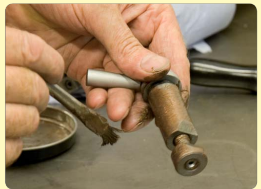
98: Assemble and grease spindle lock assembly
