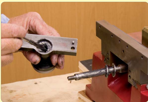
152: Grease and fit thrust bearings and bearing housing
