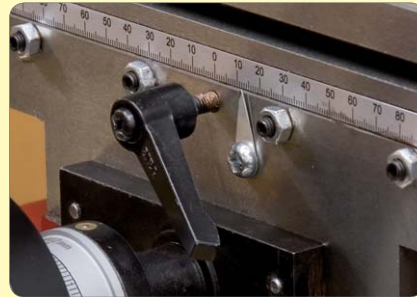
178: Wind saddle fully out and do check again
