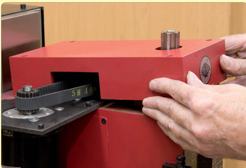
202: Fit top cover and lock down
