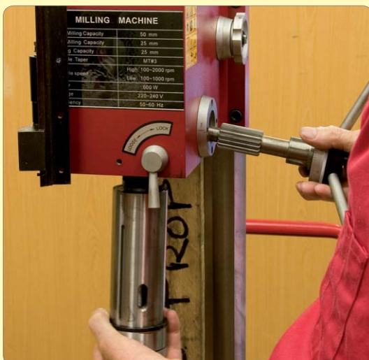
69: Holding spindle firmly, remove handle and slide spindle from bottom of housing
