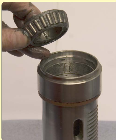
80: Grease taper roller and fit to spindle sleeve
