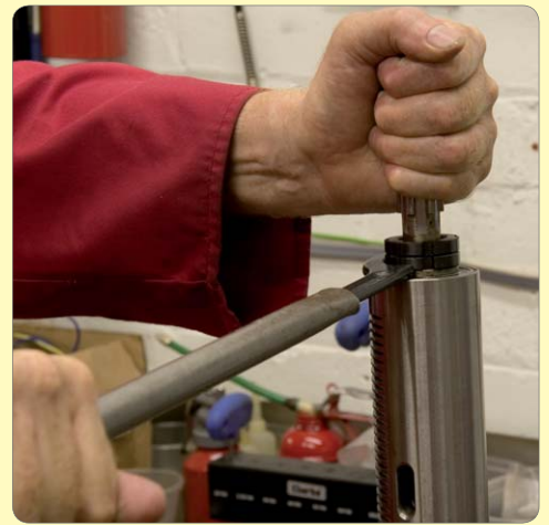
72: Hold spindle assembly in vice and remove C-Nuts and spacer
