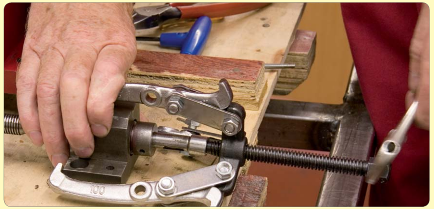
55: Remove lower thrust bearing block assembly noting orientation
