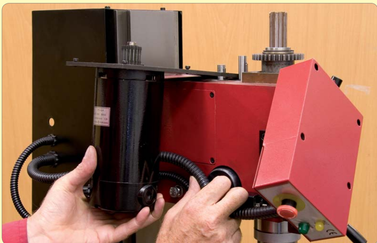
194: Fit motor and plate making sure trunking is behind motor and above bolt with locknut
