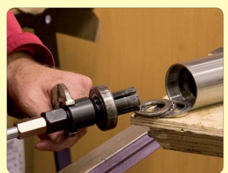
75: Using blind bearing puller, remove top ball race remove ball thrust bearing and spacer
