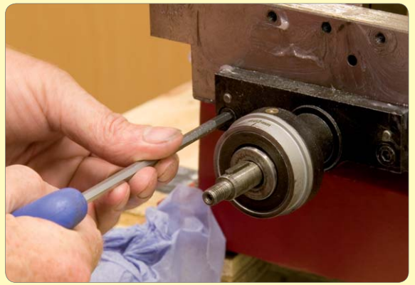
34: Remove bracket assembly screws
