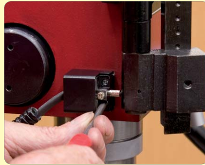
193: Fit guard micro switch and Secure trunking with P-clip
