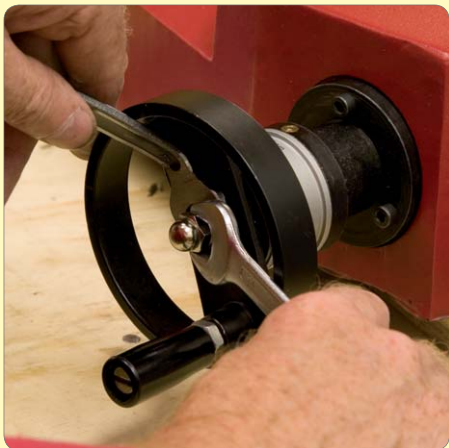
121: Fit handwheel assembly and adjust out backlash
