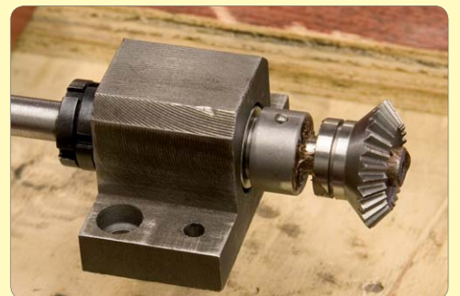
130: Slide on bevel gear leaving free to move
