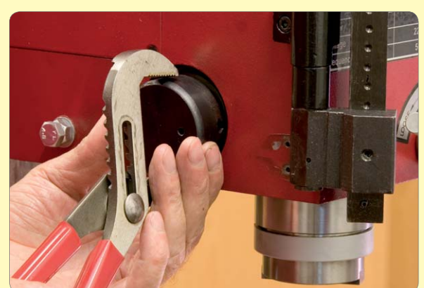
109: Fit return spring housing and turn anticlockwise to adjust tension to preference.
