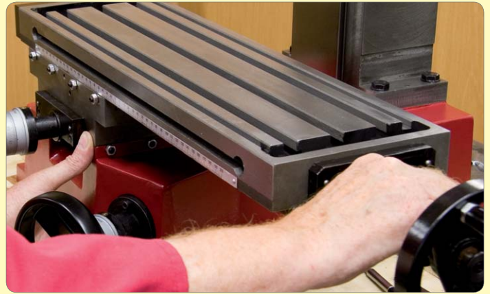
176: The same procedure as above but put thumb over joint between saddle and base - rock to and fro
