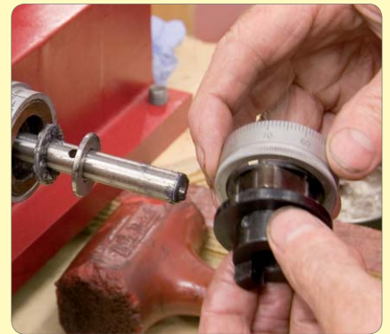
170: Grease and assemble micrometer dial with friction spring and sleeve
