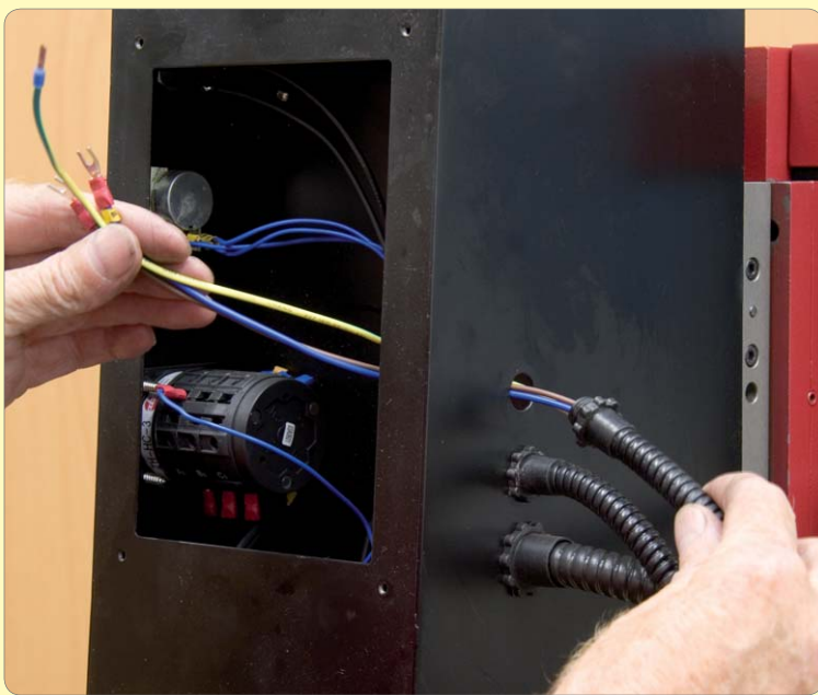
204: Thread motor wires through casing
