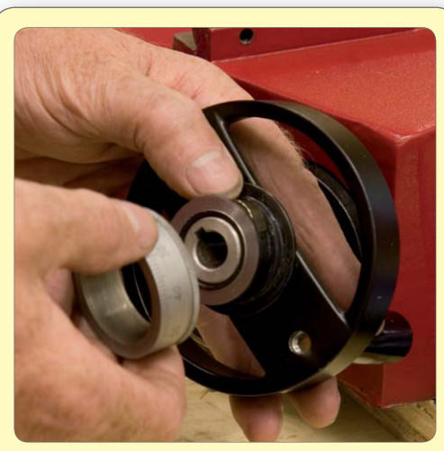
120: Grease and assemble handwheel and micrometer dial with friction spring
