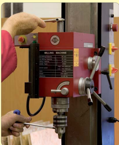
4: Loosen the drawbar...
