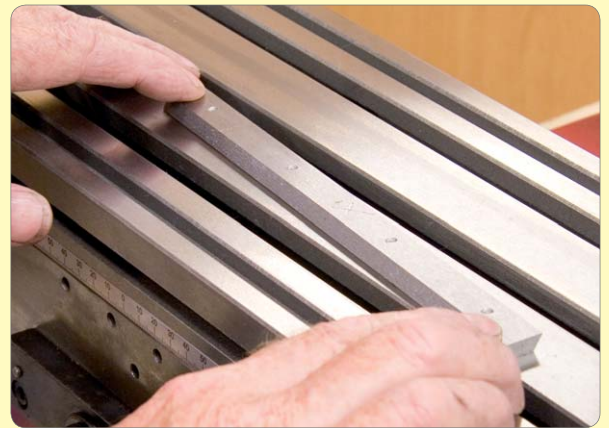
160: Check X-Axis gib strip is straight and flat
