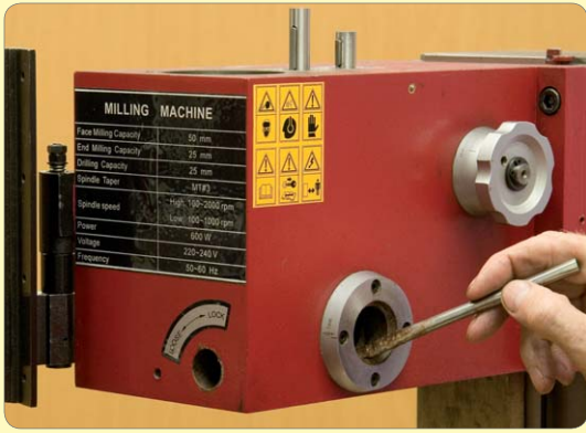
99: Grease bores for handwheel and spindle lock
