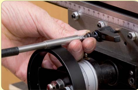
179: Fit locking levers and scale pointer
