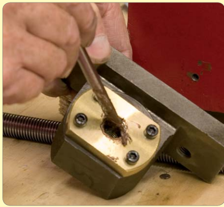
122: Grease Z-Axis nut
