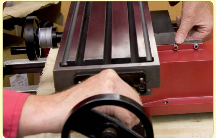
178: Wind saddle fully out and do check again
