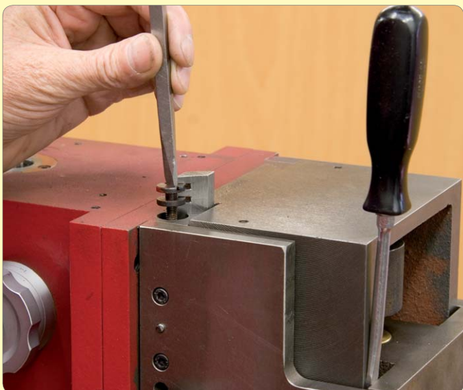
136: Wedge Z-axis nut to hold head in position and remove head gib strip
