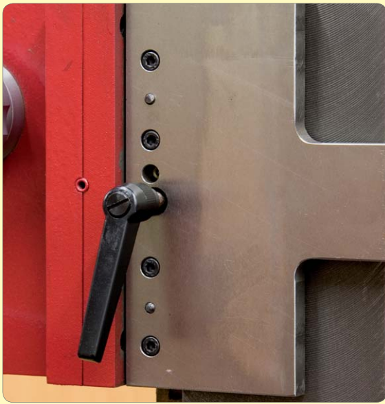
138: Fit Head locking lever
