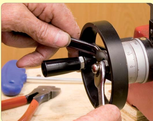
155: Fit handwheel assembly and adjust backlash
