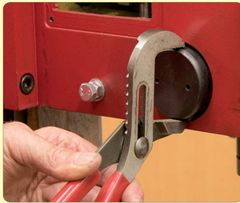
65: Remove return spring assembly carefully (see fig. 108 page 16)
