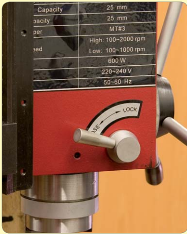
64: Lock spindle in UP position
