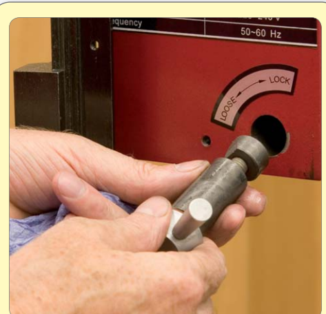
70: Remove spindle lock assembly
