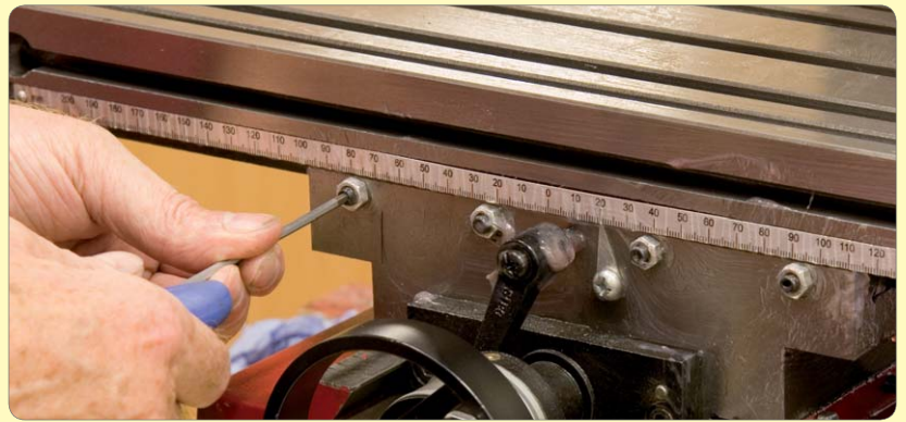
28: Slacken gib strip screws
