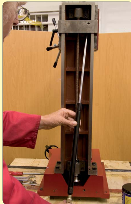
139: Fit gas strut and final adjust head gib strip
