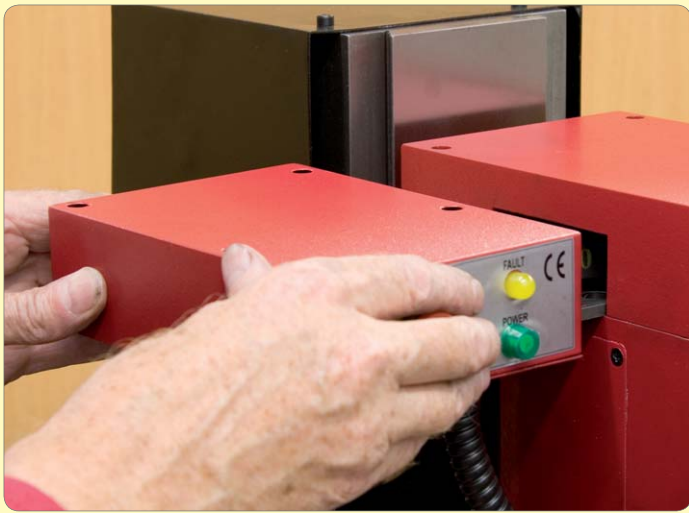
203: Fit stop switch housing - just slide on and pinch screws down
