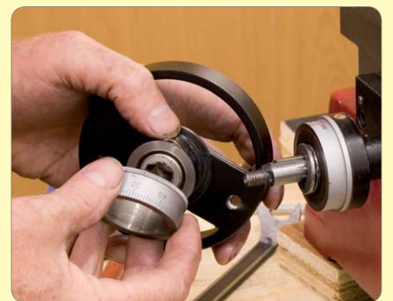
154: Grease and fit micrometer dial to handwheel with friction spring
