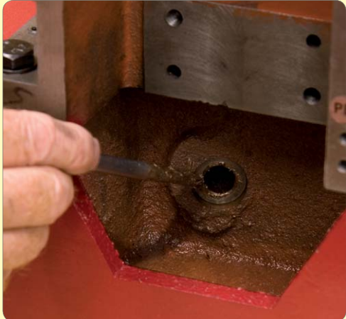
113: Grease handle shaft bore in rear of column
