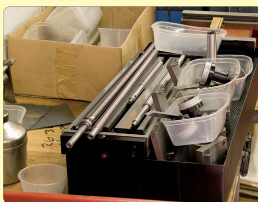
76: Wash all parts thoroughly in paraffin to remove any trace of contamination
