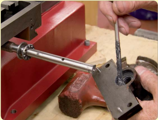
168: Grease and fit inner thrust bearing and bearing housing
