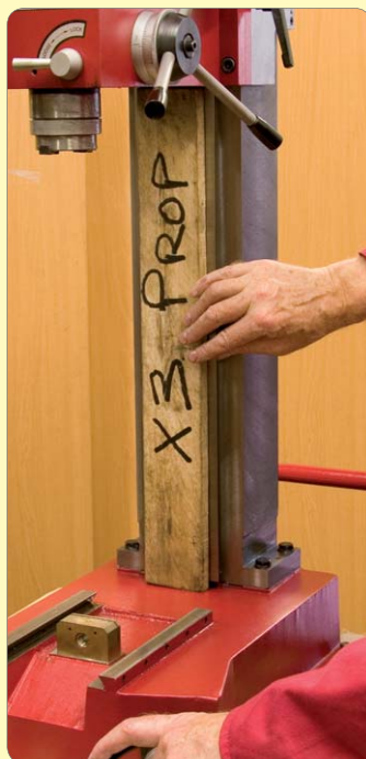
46: Place prop under head and wind down until the head just touches
